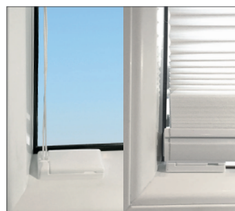
Variant: Adhesive clamping shoe on the glazing bead (depth at least 13 mm).
